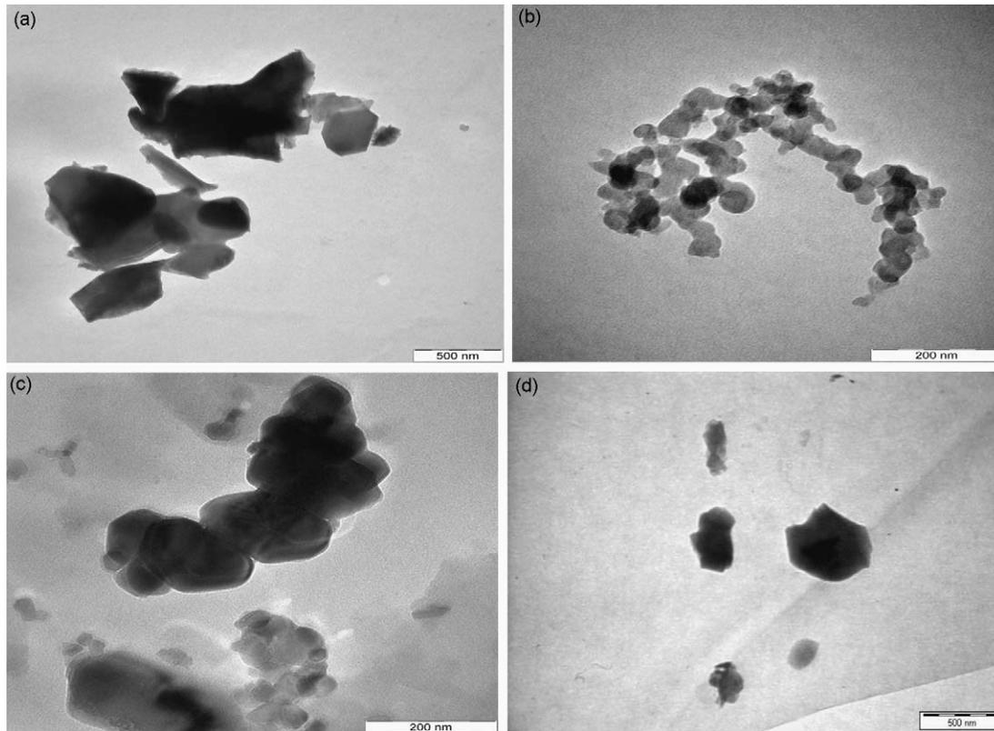
Fig. 4. TEM micrographs of the various microstructures of  $\alpha$ - $\text{Al}_2\text{O}_3$  under different conditions: (a and b) TEM micrograph of  $\alpha$ - $\text{Al}_2\text{O}_3$  in the presence of 0.1 SBDS at 24 and 48 h stirring and (c and d) TEM micrograph of  $\alpha$ - $\text{Al}_2\text{O}_3$  in the presence of 0.1 Na(AOT) at 24 and 48 h stirring.
