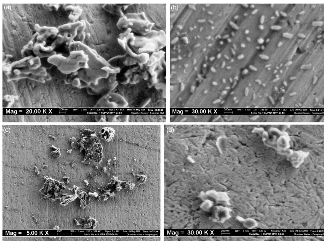
Fig. 3. SEM images of the alumina powder; (a and b) SEM micrograph of  $\alpha$ - $\text{Al}_2\text{O}_3$  in the present of 0.1 SDBS at 24 and 48 h stirring time and (c and d) SEM micrograph of  $\alpha$ - $\text{Al}_2\text{O}_3$  in the present of 0.1 Na(AOT) at 24 and 48 h stirring time.
