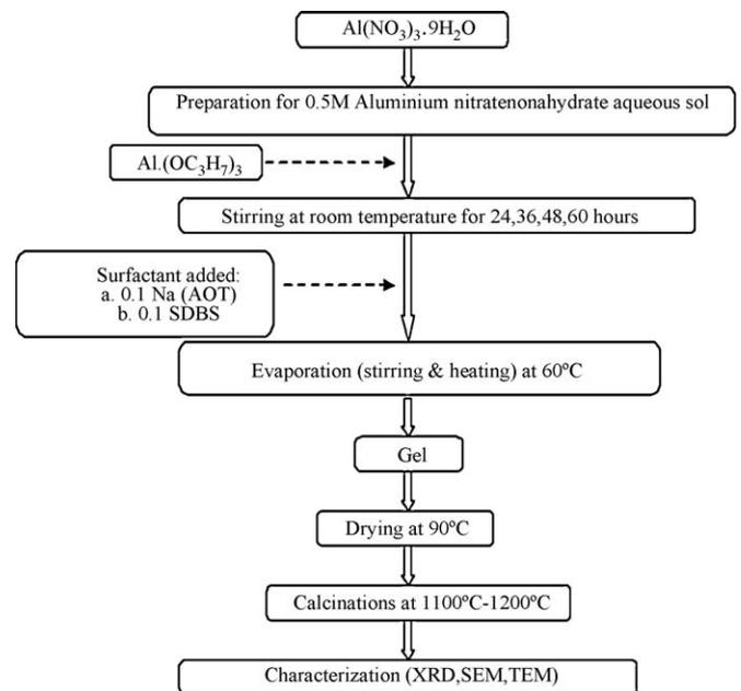
Fig. 1. Nano alumina synthesis process.
